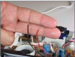
• Strip the wire half an inch using wire strippers for a 24 gauge wire.
