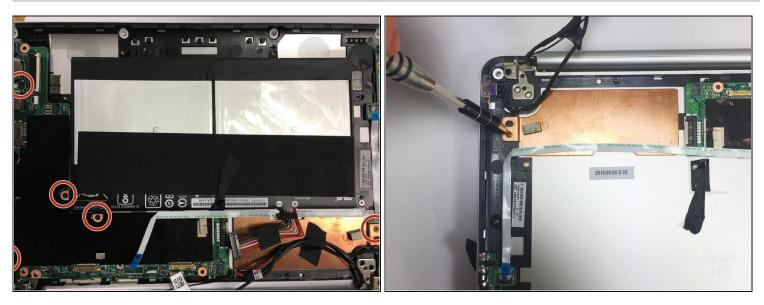
• Remove the five 2.7mm motherboard screws with a T5 screwdriver.
