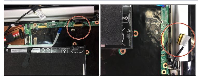
• Disconnect the digitizer board cable from the motherboard using the pointed end of a plastic spudger.
