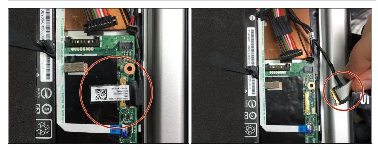
• Disconnect the LCD cable from the motherboard using the pointed end of a plastic spudger.
