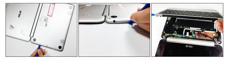
• Pry the palm rest assembly apart from the bottom cover using a spudger. This step may require extra power. Once the palm rest has been separated from the bottom cover, pull it away from the screen, rather than away from yourself.
