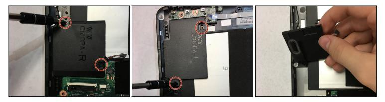
• Remove the four 4.2mm speaker screws, then remove the two speakers using a philips head screwdriver.
