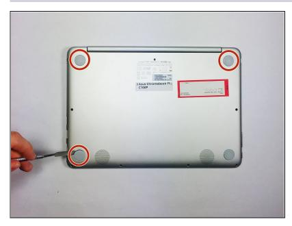
Remove three of the rubber feet on the bottom cover with a plastic or metal spudger.
