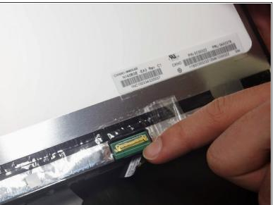
Remove the connector located at the bottom of the back of the screen.
