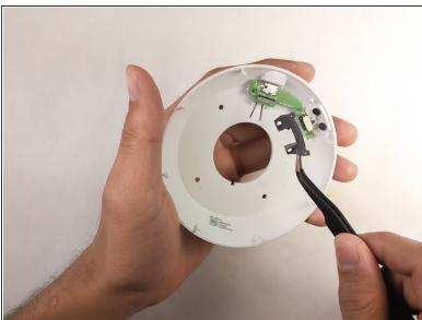
Remove the black metal plate from the board.
