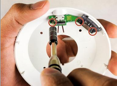
Remove the three 5.3mm T6 Torx screws from the board.
