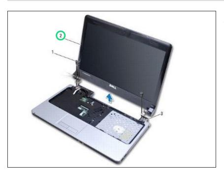
Lift and remove the display assembly from the computer base.
