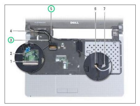
Note the routing of all the cables and remove them from their routing guides.
