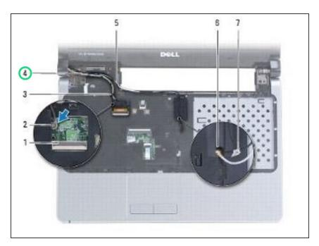
Disconnect the display cable and remove the screw from the system board.
