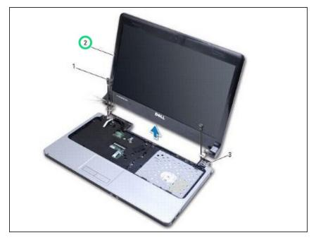
Using the alignment posts, place the NEW display assembly in position and replace the three screws that secure the display assembly to the computer base.
