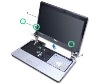
Hold the display while you remove the three screws that secure the display assembly to the computer base.
