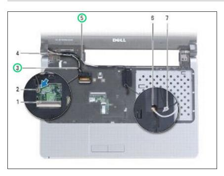
Route the Mini-Card antenna cables and display cable through their routing guides.
