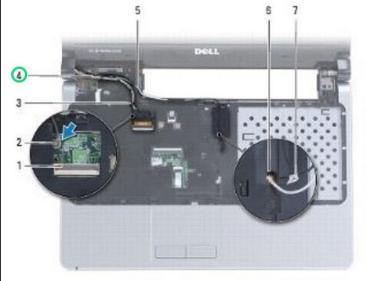
Replace the screw and connect the display cable.
