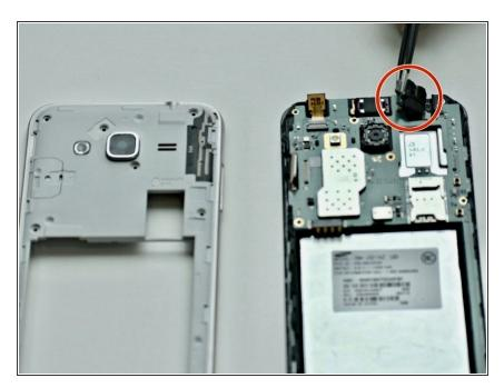
Remove the headphone jack at the top of of the phone by carefully removing it with tweezers.
