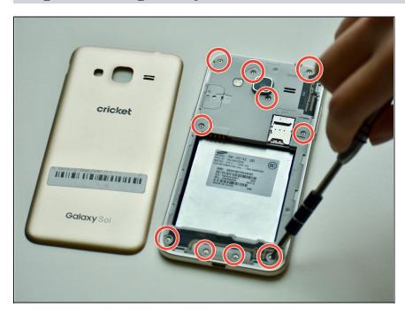
Remove the grey back of the phone by unscrewing all ten 0.4mm screws with a Phillips #00 screw bit.
