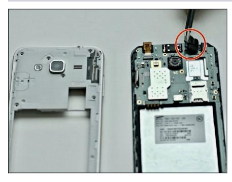
Remove the headphone jack at the top of of the phone by carefully removing it with <u>tweezers</u>.
