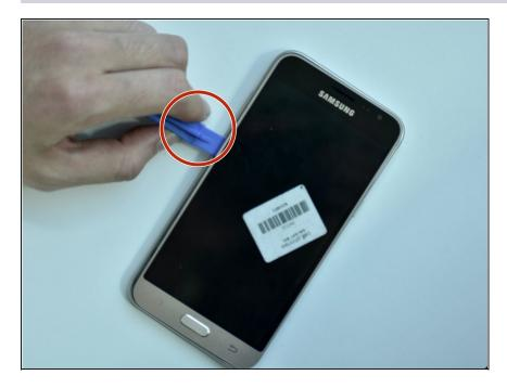
• Turn the phone around and remove the screen using the plastic tool.
