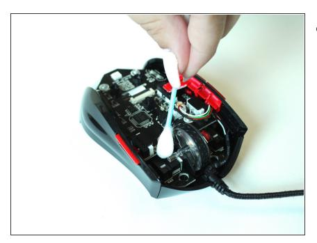
Use a Q-tip to clean around the switches.
