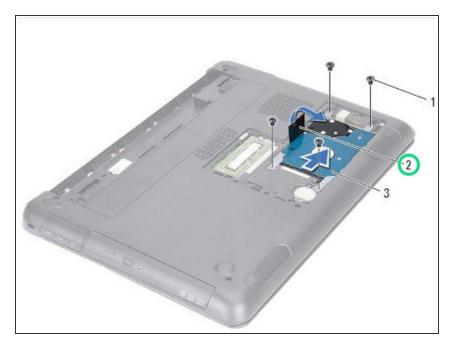
Using the pull-tab, slide the harddrive assembly into the connector on the system board.
