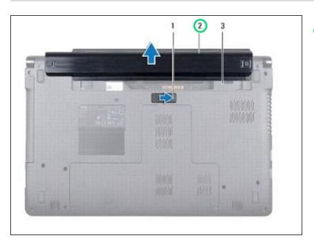
Slide the **NEW** battery into the battery bay, and push to click the battery into place.
