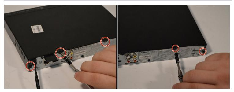
• Remove the four 5mm Phillips #1 screws that connect the black outer shell to the silver back of the device.
