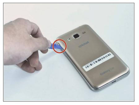
Remove the back case of the phone by using an opening tool or fingernail to lift the divot on the top left side.
