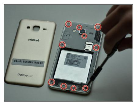
Remove all ten 0.4 mm screws with a Phillips #00 screw bit. After this, you will be able to lift up and remove the grey plastic piece.
