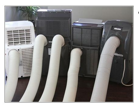
The hose is a vital piece of kit with these portable machines. There should be a series of connectors to hook to the hose. This should create an airtight seal with a little easy rotation into place. Checking that seal for a functional exhaust is essential. The tabs on the connector should then snap onto corresponding tabs on the air conditioner.
