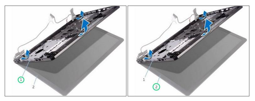
• Lift the palm-rest assembly at an angle off the display assembly.
