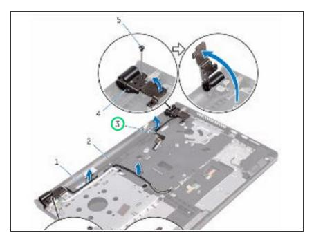
Note the display cable routing and remove the cable from its routing guides on the palm-rest assembly.
