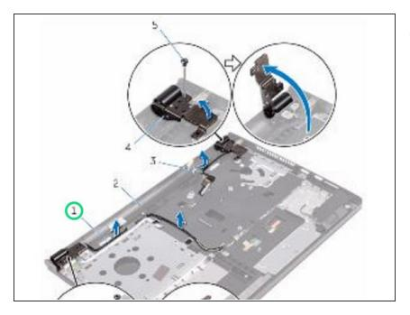
Route the antenna cables through its routing guides on the palm-rest assembly.
