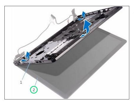
Place the NEW display assembly on the palm-rest assembly.
