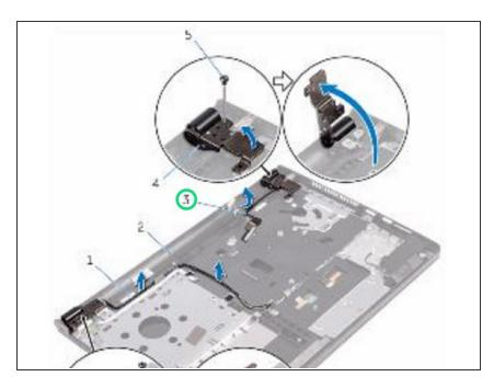
Route the display cable through its routing guides on the palm-rest assembly.
