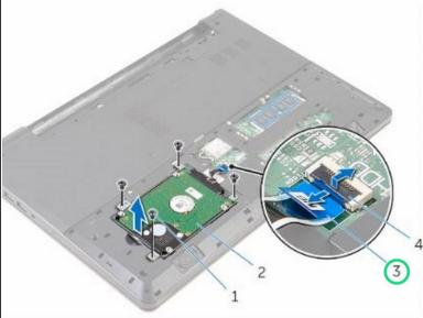
• Lift the latch and disconnect the hard-drive cable from the system board.
