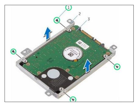
Remove the screws that secure the hard-drive bracket to the hard drive and lift the hard-drive bracket off the hard drive.
