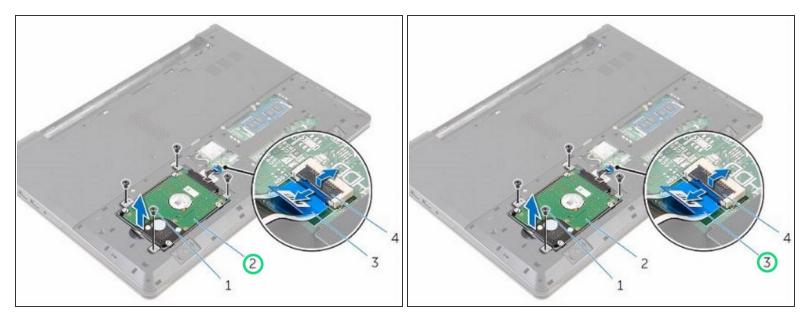
• Slide the hard-drive assembly in the computer base and align the screw holes on the hard-drive assembly with the screw holes on the computer base.
