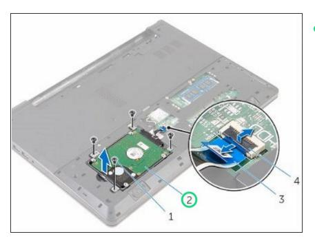
Lift the hard-drive assembly off the computer base.
