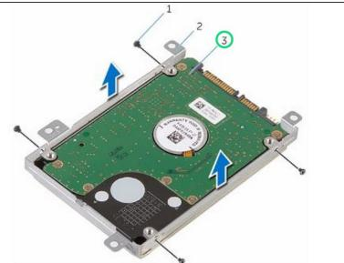
Place the hard-drive bracket over the **NEW** hard drive and align the screw holes on the hard-drive bracket with the screw holes on the hard drive.
