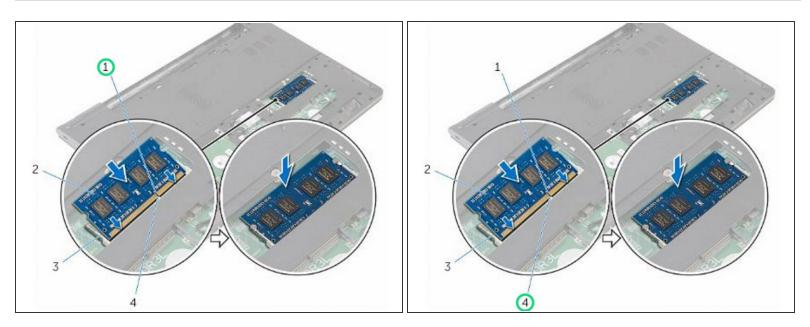
Align the notch on the NEW memory module with the tab on the memory-module slot.
