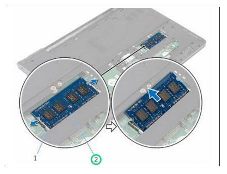
Slide and remove the memory module from the memory-module slot.
