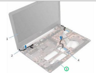
Route the display cable through its routing guides on the computer base.
