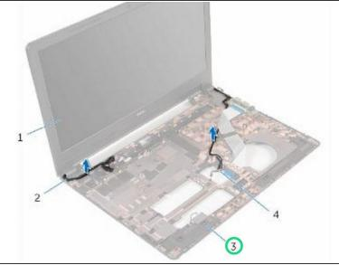
Note the antenna cable routing and remove the antenna cables from its routing guides on the computer base.
