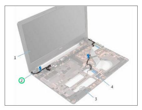
Note the display cable routing and remove the cable from its routing guides on the computer base.
