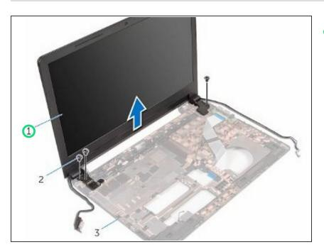
Carefully lift the display assembly off the computer base.
