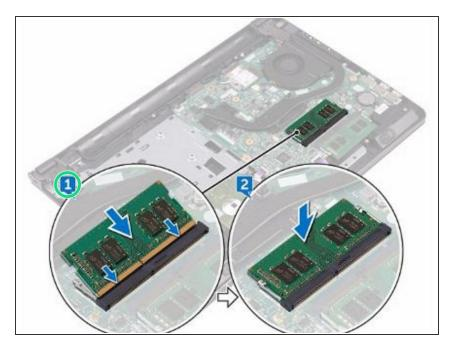
Align the notch on the memory module with the tab on the memorymodule slot and slide it firmly into the slot at an angle.
