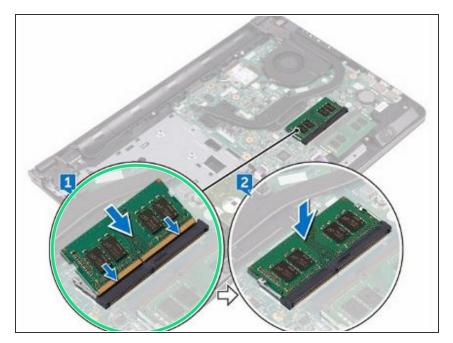
Align the notch on the NEW memory module with the tab on the memorymodule slot and slide it firmly into the slot at an angle.
