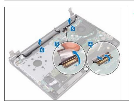
Route the display cable through the routing guides on the palm-rest assembly.
