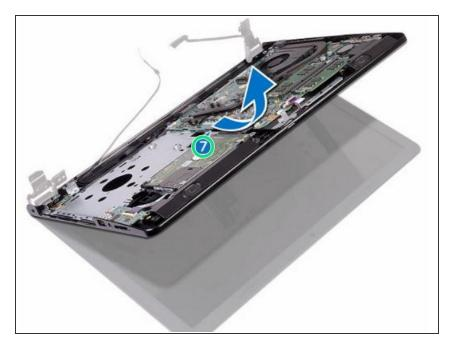
Open the palm-rest assembly at an angle and slide it off the display assembly.
