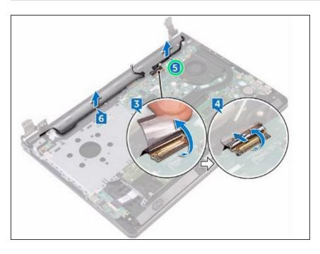
Note the antenna cable routing and remove the cable from its routing guides on the palm-rest assembly.
