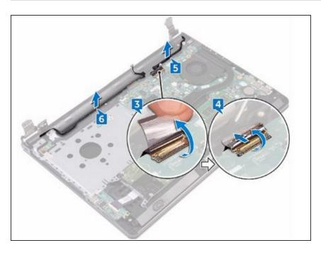
Close the display hinges and align the screw holes on the display hinges with the screw holes on the palm-rest assembly.
