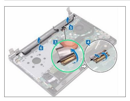
Adhere the tape that secures the display cable to the palm-rest assembly.
