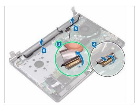
Peel the tape that secures the display cable to the palm-rest assembly.
