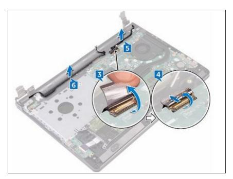
Connect the display cable and close the latch to secure the cable.
