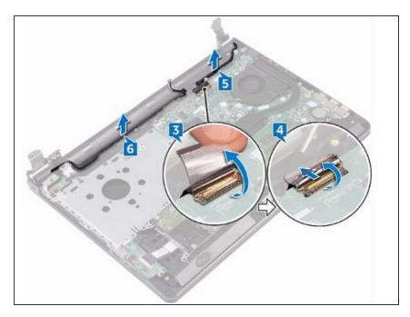
Note the display cable routing and remove the display cable from the routing guides on the palm-rest assembly.
