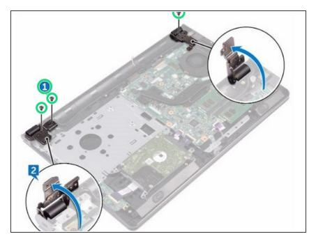
Replace the three screws (2.5x8) that secure the display hinges to the palm-rest assembly.
