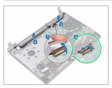
Open the latch and disconnect the display cable.
