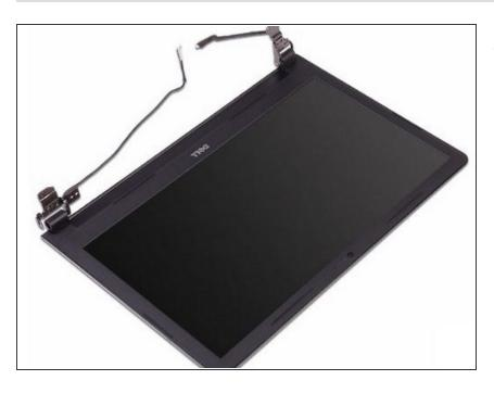
Place the **NEW** display assembly on a clean, flat surface.
