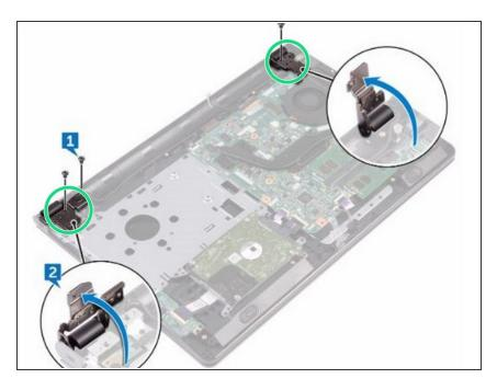
Open the display hinges to an angle of 90 degrees.
