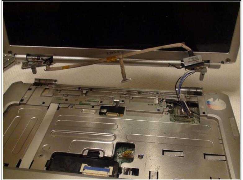
**⚠** There is a risk of dropping the lid or base of the laptop, or damaging cables. Make sure no cables are still attached.
