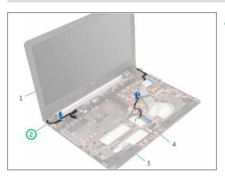
Route the display cable through its routing guides on the computer base.
