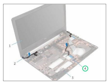
Route the antenna cables through its routing guides and slide the antenna cables through the slot on the computer base.
