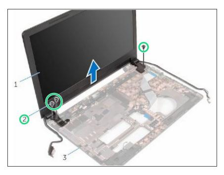
Remove the screws that secure the display hinges to the computer base.
