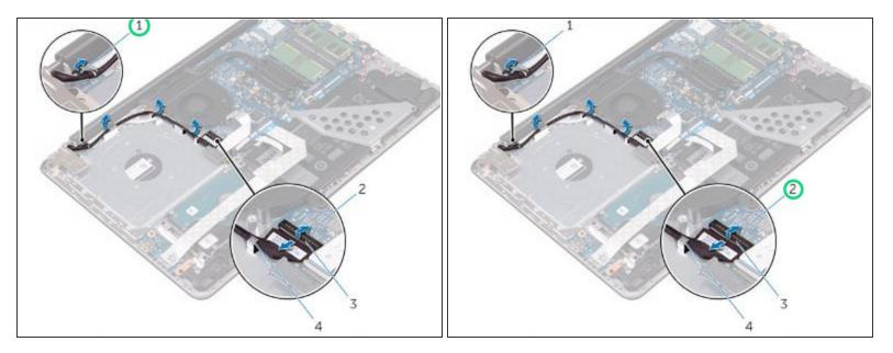
Slide the display cable to the connector on the system board and close the latch to secure the cable.
