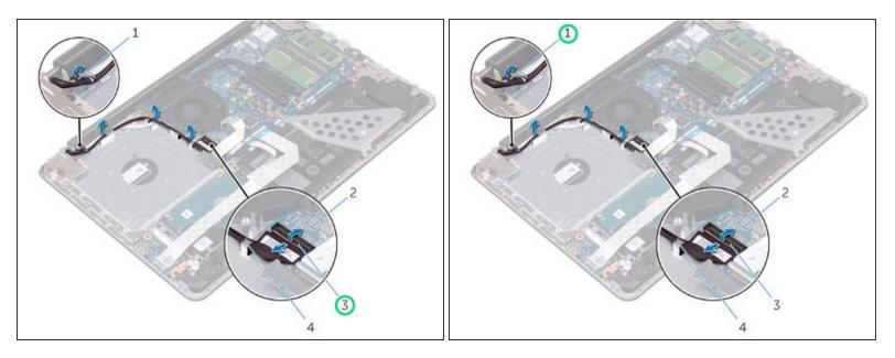
Lift the latch and disconnect the display cable from the system board.
