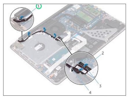
Note the display cable routing and remove the cable from its routing guides.
