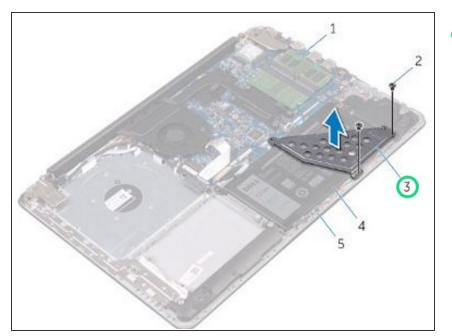
• Lift and remove the battery bracket.
