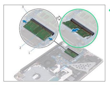
• Remove the memory module from the memory-module slot.
