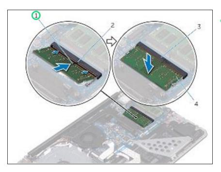
Align the notch on the NEW memory module with the tab on the memorymodule slot.
