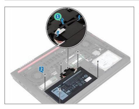
Route the battery cable through the routing guides on the computer base.
