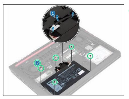
Replace the five screws (M2x5 T8) that secure the battery to the computer base.
