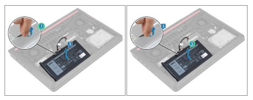
Using the pull tab, lift the battery, along with its cable, off the computer base.
