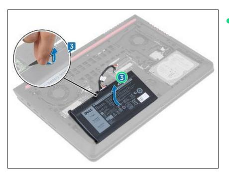
Slide the **NEW** battery in the slot on the computer base.
