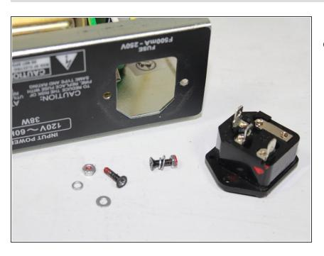
Pull the power input jack out of the mounting bracket. Once the old power jack is removed, to install the replacement power jack, follow the guide in reverse.
