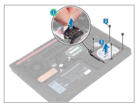
• Connect the hard-drive cable to the connector on the system board.
