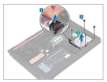
Lift the hard-drive assembly, along with its cable, off the computer base.
