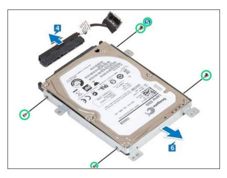
Replace the four screws (M3x3) that secure the hard-drive bracket to the hard drive.
