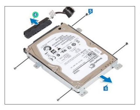
Disconnect the interposer from the hard-drive assembly.
