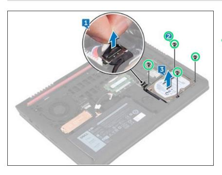
Remove the four screws (M2x5) that secure the hard-drive assembly to the computer base.
