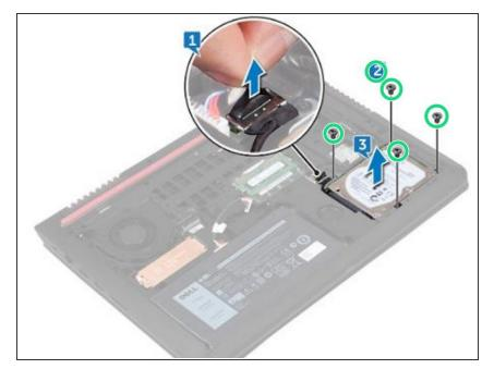
Remove the four screws (M3x3) that secure the hard-drive bracket to the hard drive.
