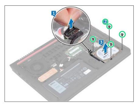
Align the screw holes on the harddrive assembly with the screw holes on the computer base.
