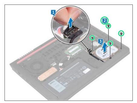
Replace the four screws (M2x5) that secure the hard-drive assembly to the computer base.
