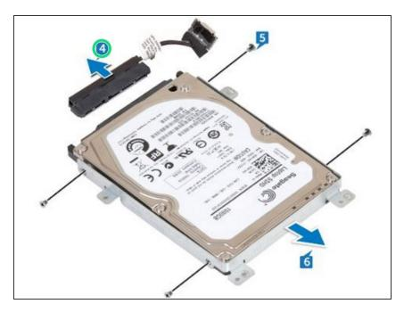
Connect the interposer to the harddrive assembly.
