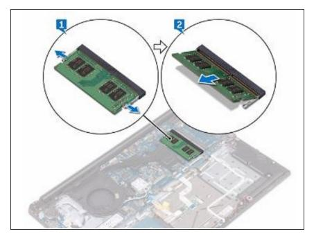
Align the notch on the memory module with the tab on the memorymodule slot.
