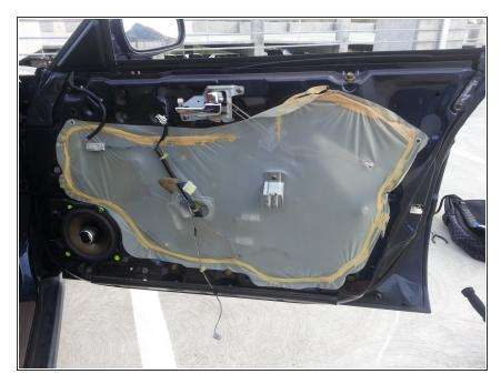
Remove the interior door panel completely, exposing the inside of the door and the front speaker.
