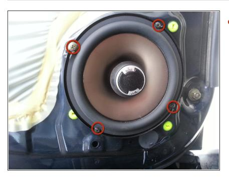
Remove the four screws holding the front door speaker in.
