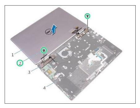
Remove the screws that secure the display assembly to the palm-rest assembly.
