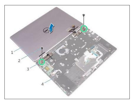
With the display facing down, align the screw holes on the display hinges with the screw holes on the palm-rest assembly.
