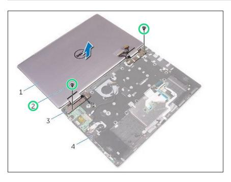
Replace the screws that secure the NEW display assembly to the palmrest assembly.
