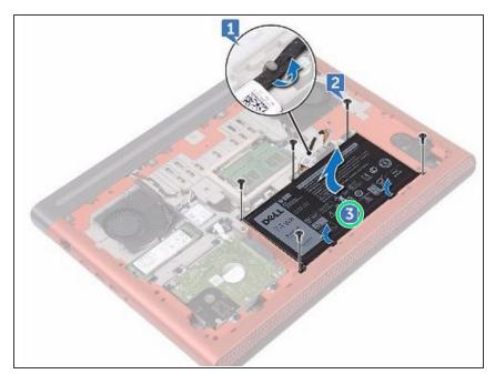
Slide the **NEW** battery in the slot on the computer base and align the screw holes on the battery with the screw holes on the computer base.
