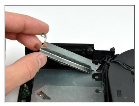
Maneuver the metal bracket near the speaker out of the internal frame.
