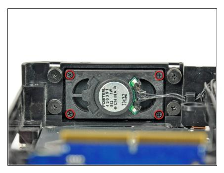
Remove the four Phillips screws securing the speaker to its metal bracket.
