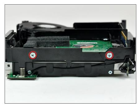
Remove the two Phillips screws securing the side of the hard drive to the internal frame.
