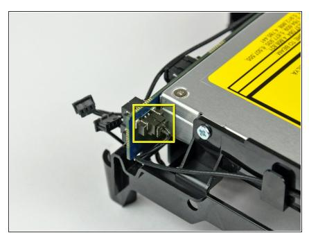
Use a pair of tweezers or your fingernails to disconnect the speaker cable connector from the interconnect board.
