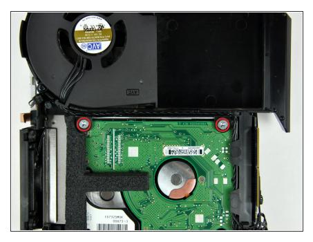
Remove the two Phillips screws securing the bottom of the hard drive to the internal frame.
