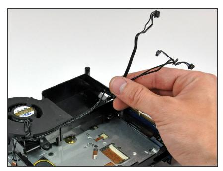
De-route the cables from the channel in the internal frame until the speaker cable is free.
