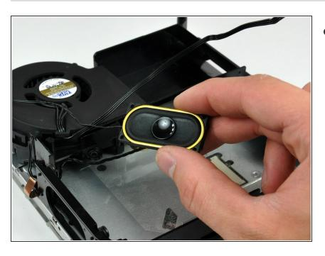
Lift the speaker out of the internal frame.
