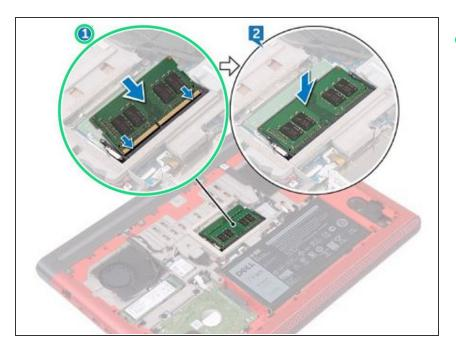
Align the notch on the NEW memory module with the tab on the memorymodule slot and slide it firmly into the slot at an angle.
