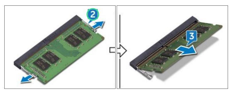
• Use your fingertips to carefully spread apart the securing-clips on each end of the memory-module slot until the memory module pops up.
