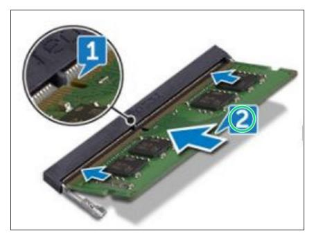
Slide the memory module firmly into the slot at an angle.
