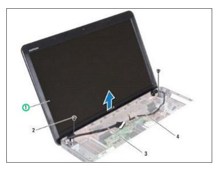
Place the **NEW** display assembly in position and replace the two screws (one on each side) that secure the display assembly to the computer base.
