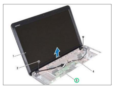
Route the display cable into the routing guide and connect the display cable to the connector on the system board.
