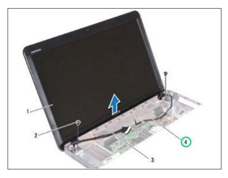
Make a note of the Wireless Mini-Card antenna cable routing and disconnect the Wireless Mini-Card antenna cable from the Wireless Mini- Card.
