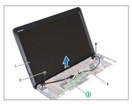
Disconnect the display cable from the connector on the system board and remove it from the routing guide.
