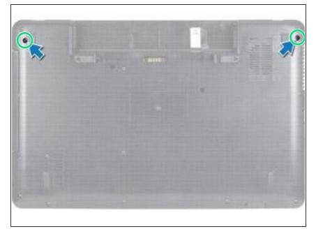
Turn the computer over and replace the two screws at the base of the computer.
