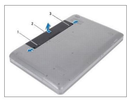
Align the tabs on the NEW battery with the slots on the battery bay.
