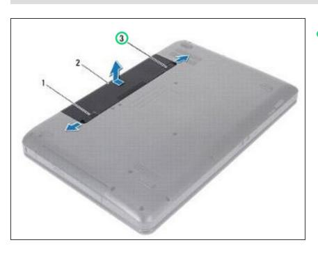
Slide the battery lock latch to the unlock position.
