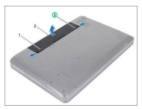
Slide the battery lock latch to the lock position.
