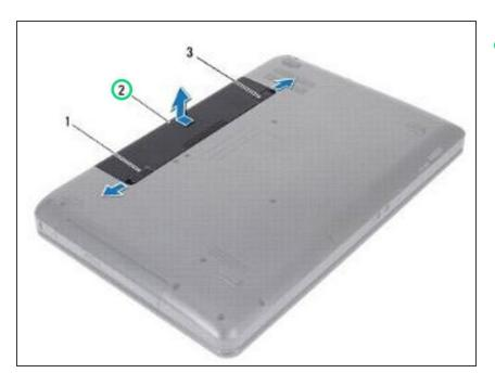
Slide the battery into the battery bay until it clicks into place.
