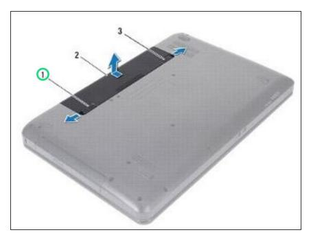
Slide the battery release latch to the side.
