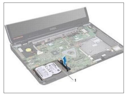
Align the hard-drive assembly with the connector on the system board and press the hard-drive assembly into the hard-drive bay until it is fully seated.
