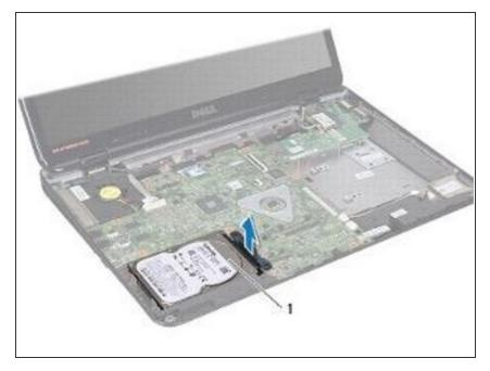
Turn the computer over and lift the hard-drive assembly out of the harddrive bay to disconnect the harddrive assembly from the connector on the system board.
