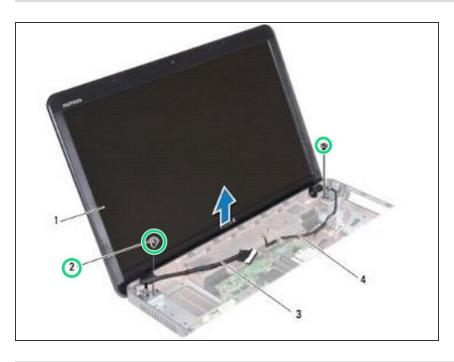
Turn the computer over and replace the two screws at the base of the computer.
