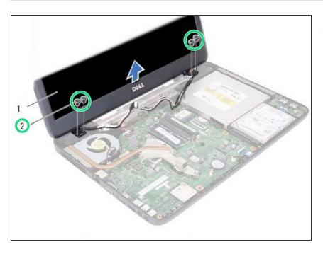
Remove the four screws (two on each side) that secure the display assembly to the computer base.
