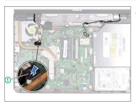
Disconnect the display cable from the connector on the system board.
