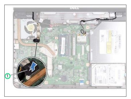
Connect the display cable to the connector on the system board.
