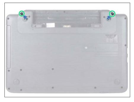
Replace the two screws to the computer base.
