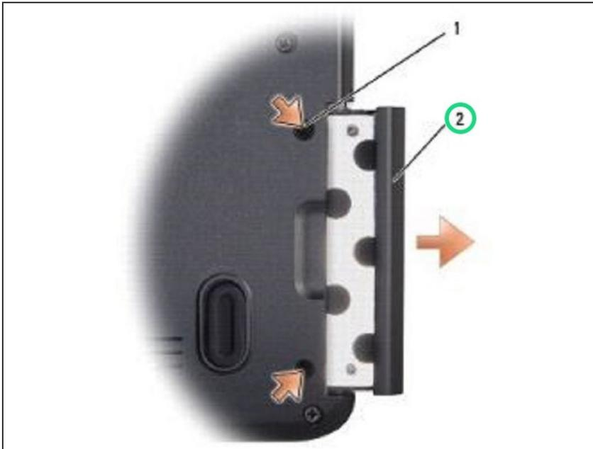
★ NOTICE: Use firm and even pressure to slide the hard drive into place. Excessive force may result in damage to the connector.
