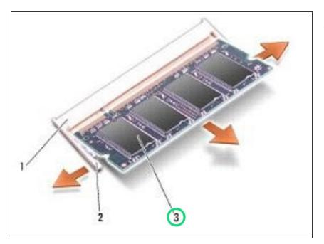
• Remove the memory module from the connector.
