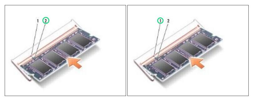
Align the notch in the edge of the NEW memory module with the tab in the memory module connector.
