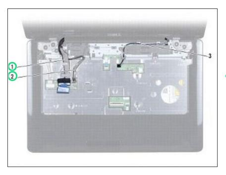
Disconnect the display cable and camera cable from the respective system board connectors and
