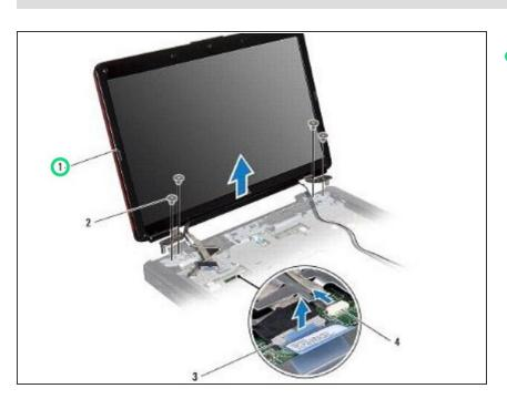
Lift and remove the display assembly from the computer base.
