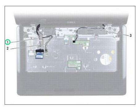
Route the display cable and camera cable into their routing guides and connect the cables to the respective system board connectors.
