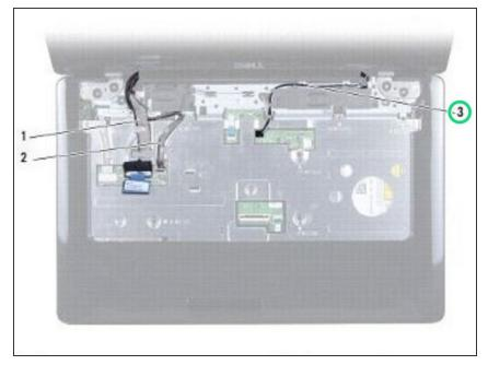
Route the Mini-Card antenna cables, and guide the cables to the bottom of the computer through the cable routing slot.
