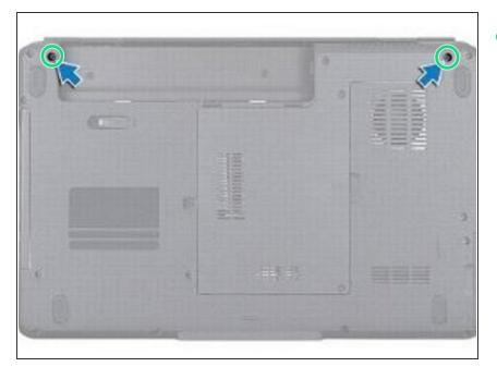
Replace the two screws at the bottom of the computer.
