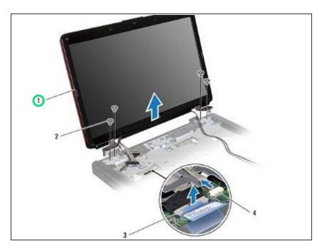
Place the display assembly in position and replace the four screws that secure the display assembly to the computer base.
