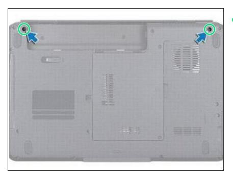
Remove the two screws from the computer base.
