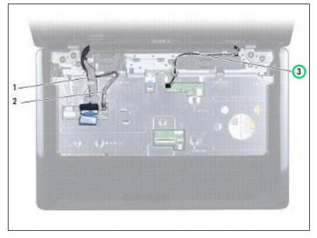
Make note of the Mini-Card antenna cable routing and carefully dislodge the antenna cables from the cable routing slot on the computer. Pull the cables away, so that they are clear of the palm rest.
