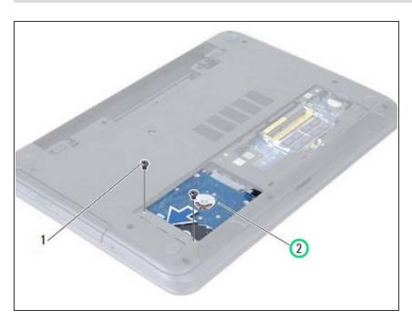
Slide the hard-drive assembly forward to disconnect the hard-drive assembly from the system board.
