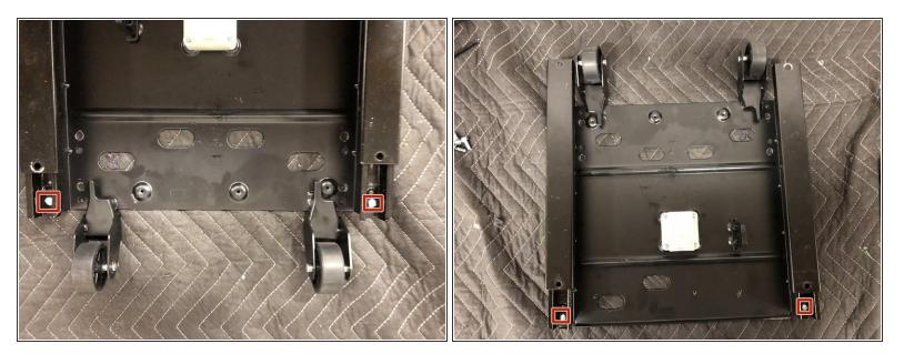
Remove the final 4 screws holding the slides in place.
