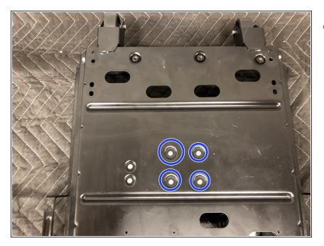
If the Feed Screw Nut needs to be replaced remove these 4 screws. They are held in by nuts that may need to be held when removing the screw
