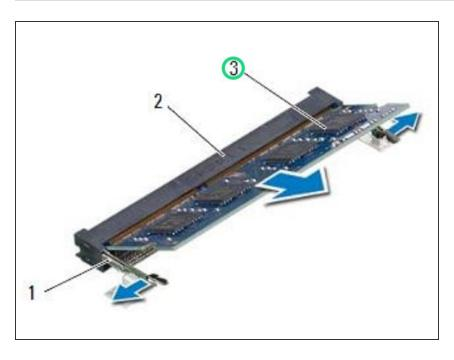
Remove the memory module from the memory-module connector.
