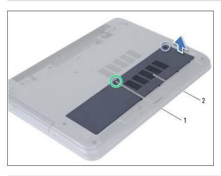
Tighten the captive screw that secures the memory-module cover to the computer base.
