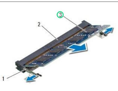
• Use your fingertips to carefully spread apart the securing clips on each end of the memory-module connector until the memory module pops up.
