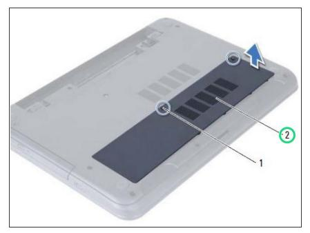
Slide the tabs on the memorymodule cover into the slots on the computer base and snap the memory-module cover into place.
