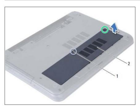
Using your fingertips, lift the memory-module cover out of the slots on the computer base.
