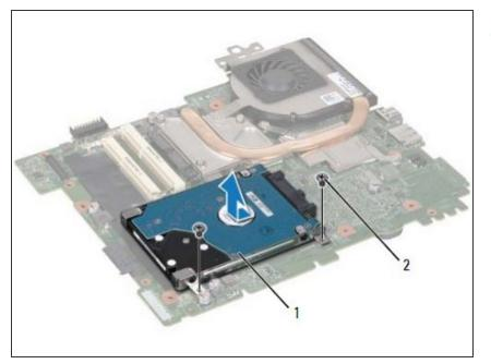
Slide the hard-drive assembly to connect it to the system-board connector.
