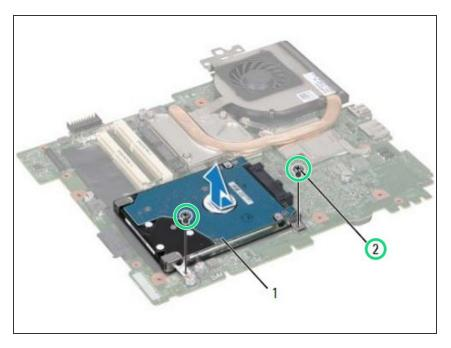
Replace the two screws that secure the hard-drive assembly to the system-board.
