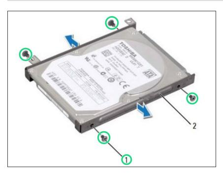
Remove the four screws that secure the hard drive to the hard-drive bracket.
