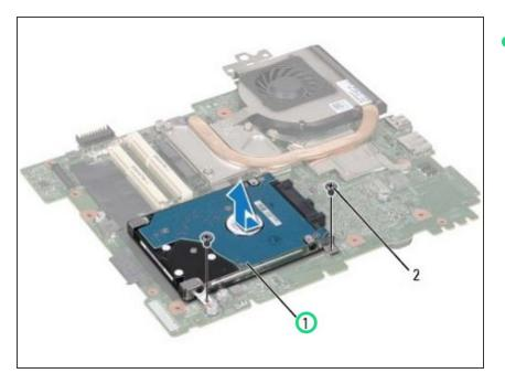
Lift the hard-drive assembly off the system board.
