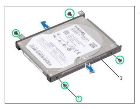
Replace the four screws that secure the hard drive to the hard-drive bracket.
