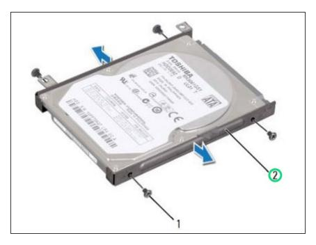
• Lift the hard drive away from the hard-drive bracket.
