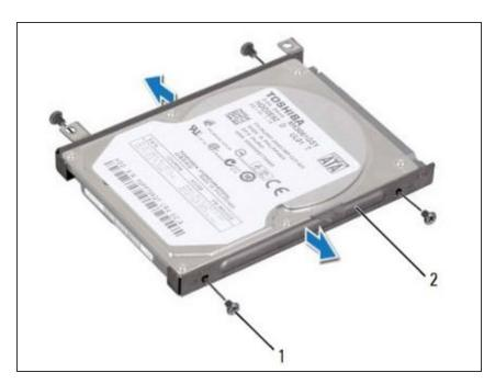
Place the **NEW** hard drive in the hard-drive bracket.
