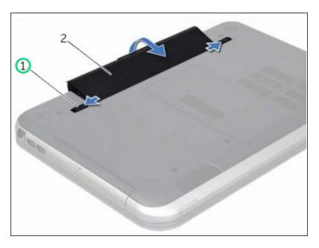
Slide the battery release latches to the unlock position.
