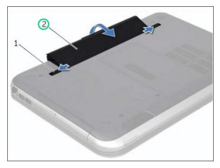
Lift the battery out of the battery bay.
