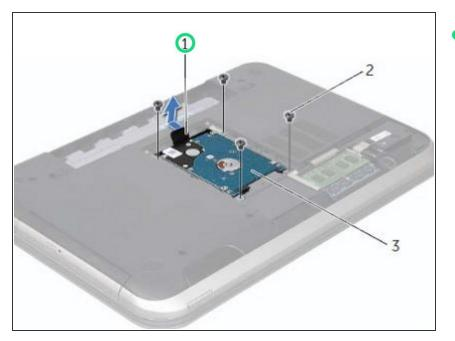
Using the pull-tab, slide the harddrive assembly toward the front of the computer, to connect the harddrive assembly to the connector on the system board.
