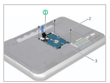
Using the pull-tab, slide the harddrive assembly toward the back of the computer to disconnect the hard-
