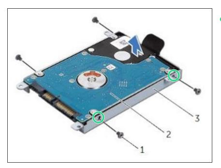
Align the screw holes on the hard drive-bracket with the screw holes on the **NEW** hard drive.
