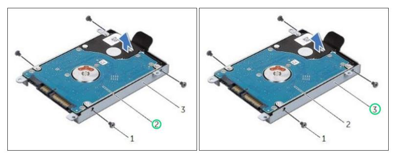
• Lift the hard drive off the hard-drive bracket.
