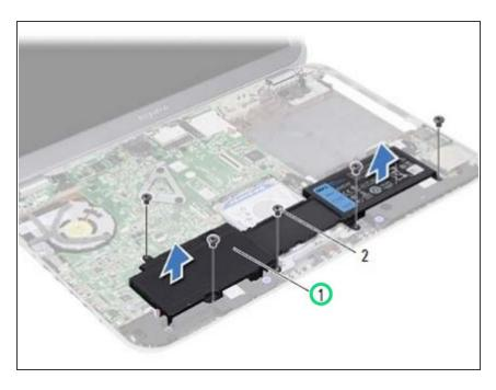
Lift the battery to disconnect it from the system board and remove the battery from the computer base.
