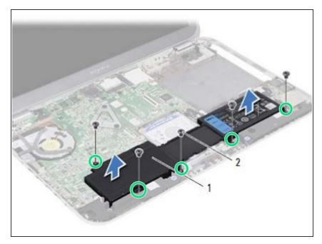
Align the screw holes on the NEW battery with the screw holes on the computer base and press down on the battery connector.
